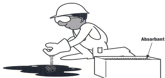
▼ Figure 2-19. Always Clean Up Oil Leaks Immediately
