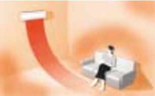
During heating the near-vertical flaps direct air to the floor to quickly warm the room.
