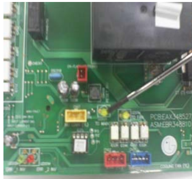
communication connector & LED in inverter compressor PCB
