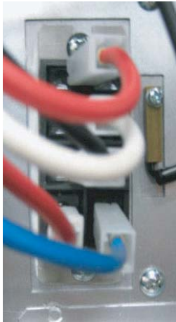
* Inverter PCB & bridge diode wiring
