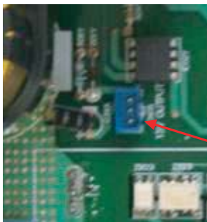
15V input power on Inverter PCB
