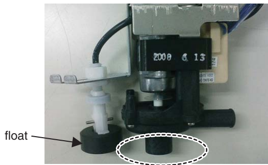
A:Point to check rotating
