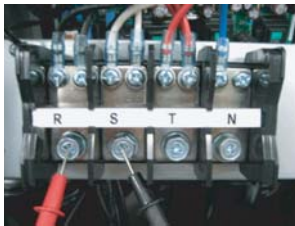
* Measuring input voltage
