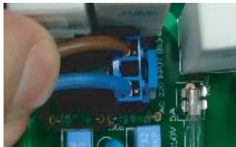
Inverter PCB assembly power connection
