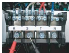
* Measuring input voltage
