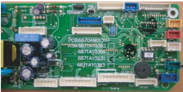
← CN-REMO : Remote controller connection
