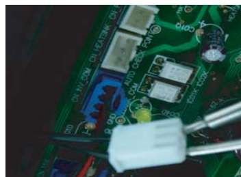
Checking temperature sensor disconnection
