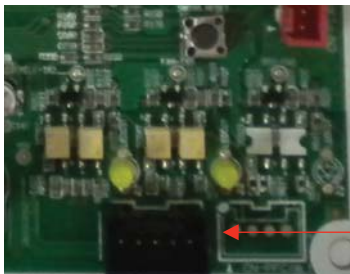
15V Input power on Inverter PCB
