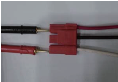
* Fan Motor resistance measuring between each phase
