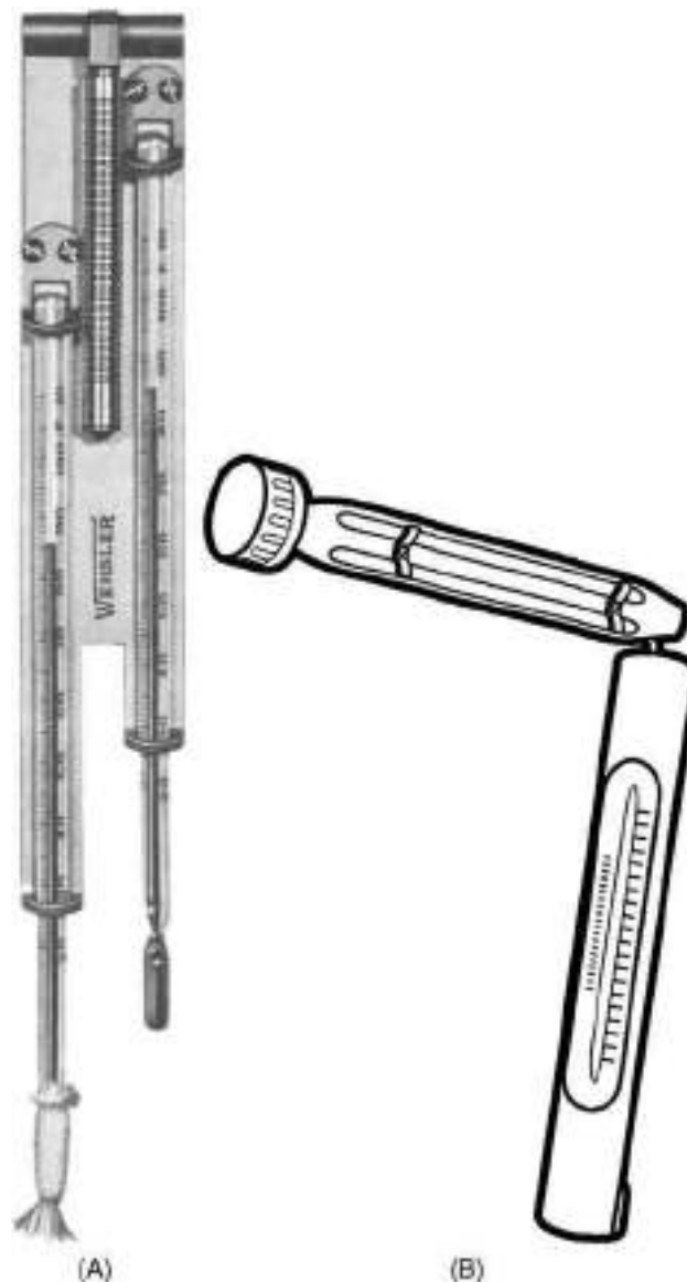
FIGURE 11.8 (A) Wet-bulb and dry-bulb thermometers mounted together. Note the knurled and ringed rod between the two at the top of the scales. It is used to hold the unit and twirl it in the air. (B) Bacharach sling psychrometer. ( Weksler )
