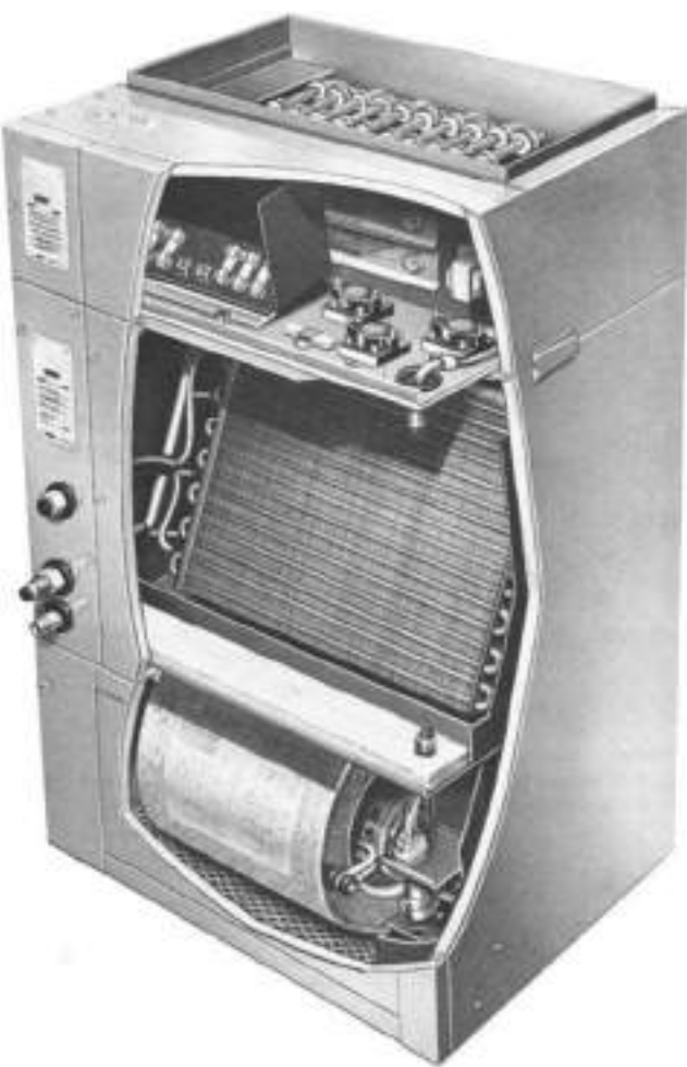
FIGURE 5.8 This unit fits in small closets or corners. It is capable of producing hot water or electric heat as well as cooling. Note the heating coils on the top of the unit. It comes in three sizes, 1.5, 2, and 2.5 tons. ( Lennox )
