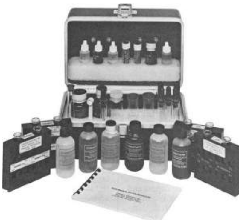
FIGURE 8.1 Field kit for testing pH, phosphate, chromate, total hardness, calcium hardness, alkalinity, and chloride. ( Virginia Chemicals )
