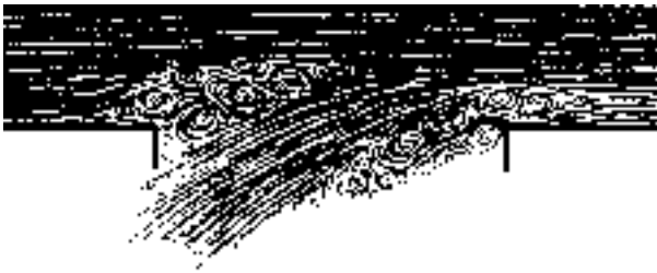
FIGURE 9.6 This flow path diagram shows the pronounced one-sided flow effect from an outlet opening before the corrective effect of air-turning devices. ( Tuttle & Bailey )
